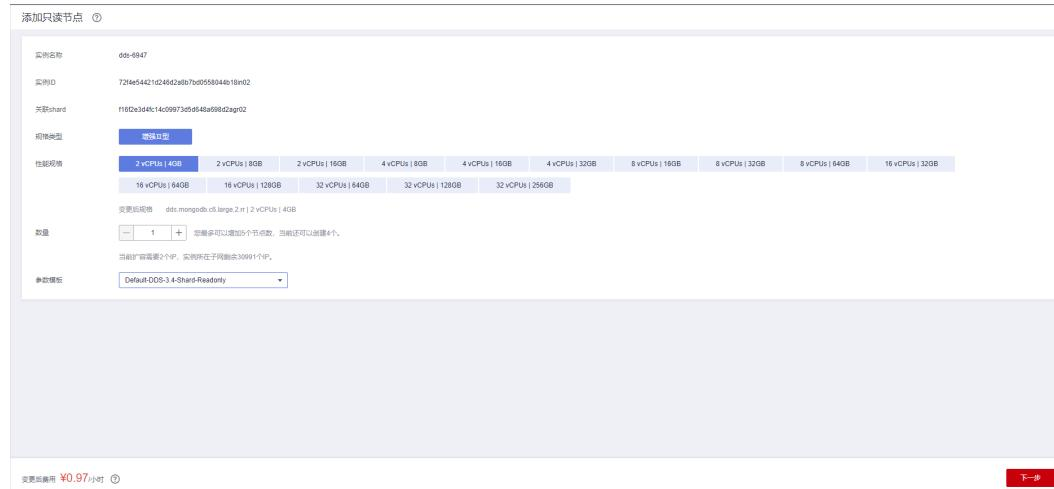
The screenshot shows the 'Add Read Node' configuration page. It includes fields for '实例名称' (Instance Name), '实例ID' (Instance ID), '关联shard' (Associated Shard), '规格类型' (Specification Type) set to '增强机型' (Enhanced Model), '性能规格' (Performance Specification) set to '2 vCPUs | 4GB', '数量' (Quantity) set to 1, and '参数模板' (Parameter Template) set to 'Default-DDS-3.4-Shard-Ready'. A note at the bottom states '变更后费用 ¥0.97 小时' (Change cost after 0.97 hours).
