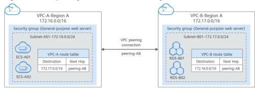
Figure 5-1 VPC peering connection network diagram
