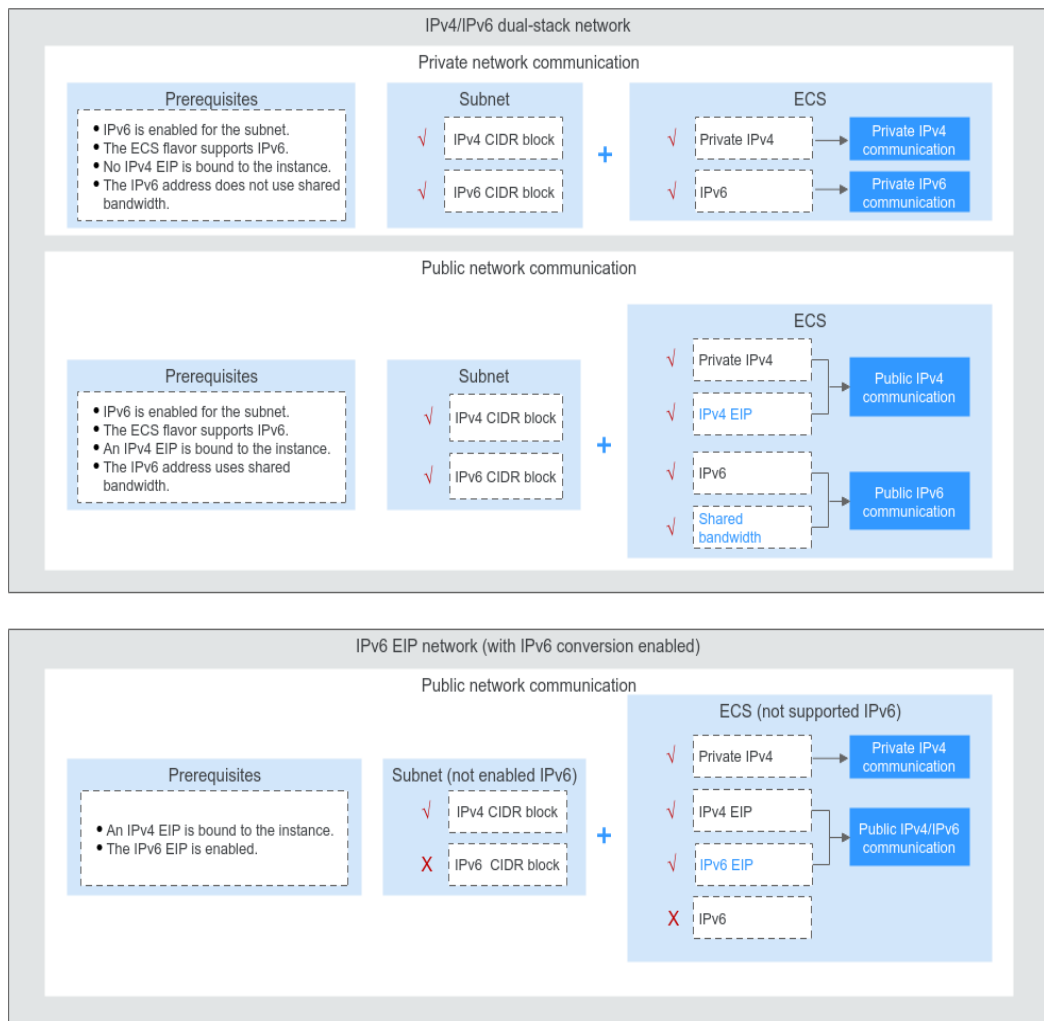
Figure 13-5 Application scenarios and resource planning of IPv6 networks
