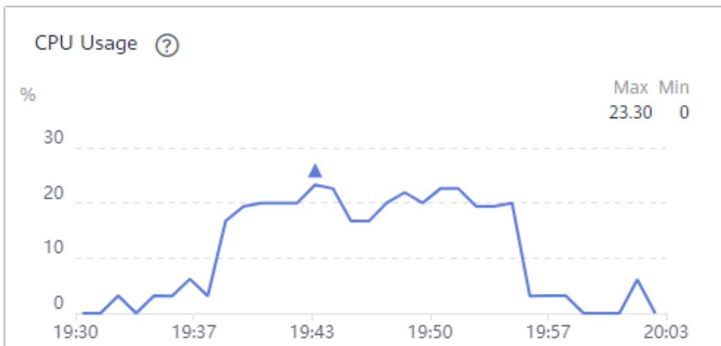
Figure 12-6 broker-2 CPU usage (batch.size = 16 KB)
