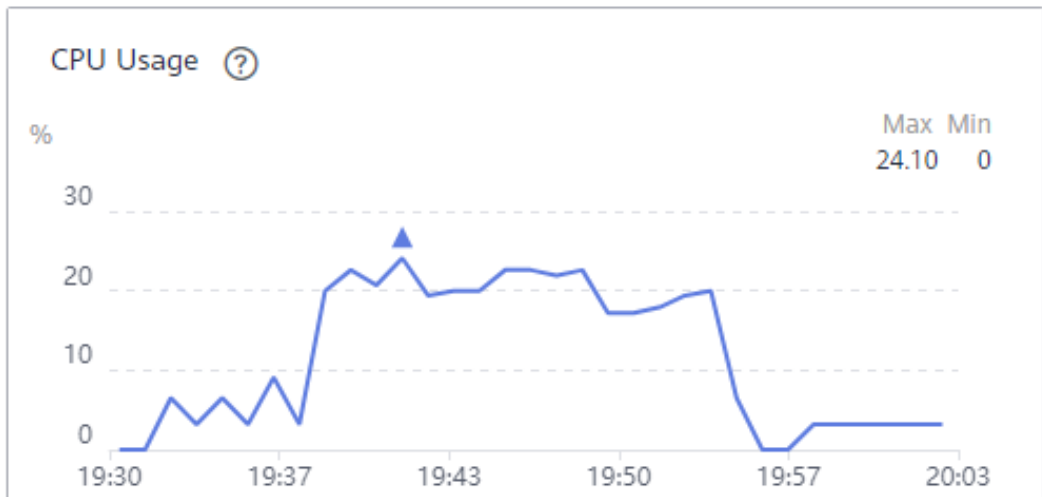
Figure 12-2 broker-0 CPU usage (batch.size = 16 KB)
