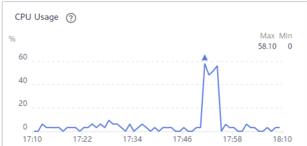
Figure 12-1 broker-0 CPU usage (batch.size = 1 KB)
