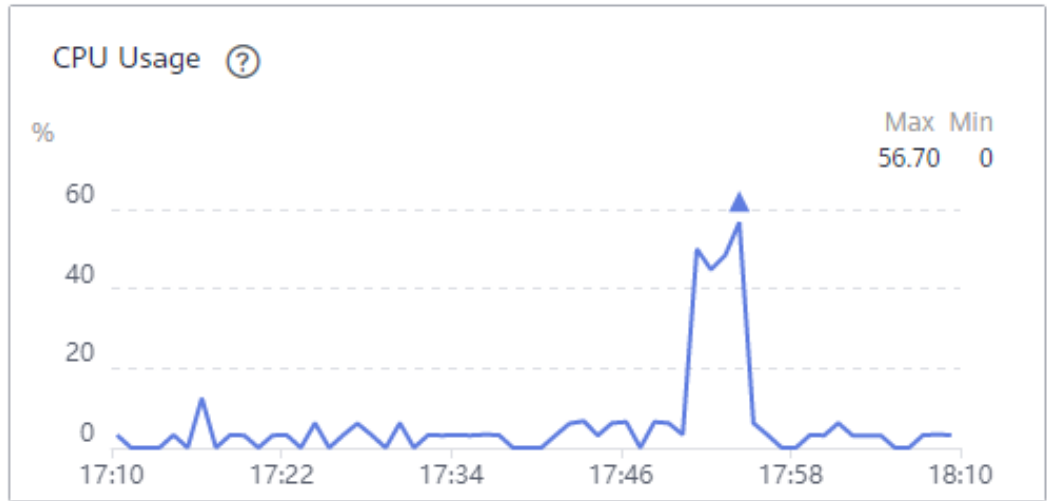
Figure 12-3 broker-1 CPU usage (batch.size = 1 KB)
