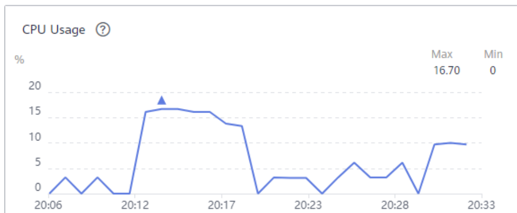
Figure 12-10 broker-1 CPU usage (different AZs)
