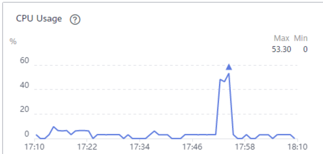
Figure 12-5 broker-2 CPU usage (batch.size = 1 KB)
