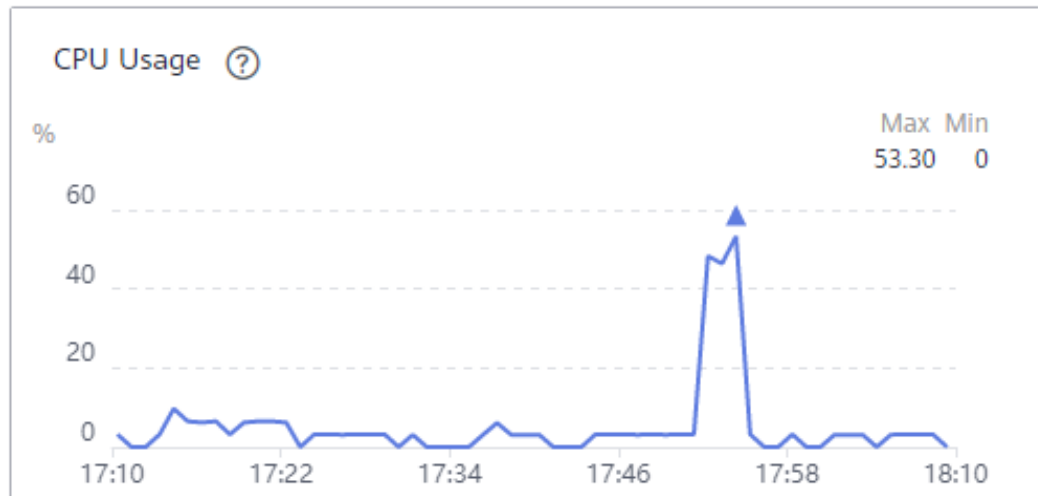
Figure 12-17 broker-2 CPU usage (one replica)
