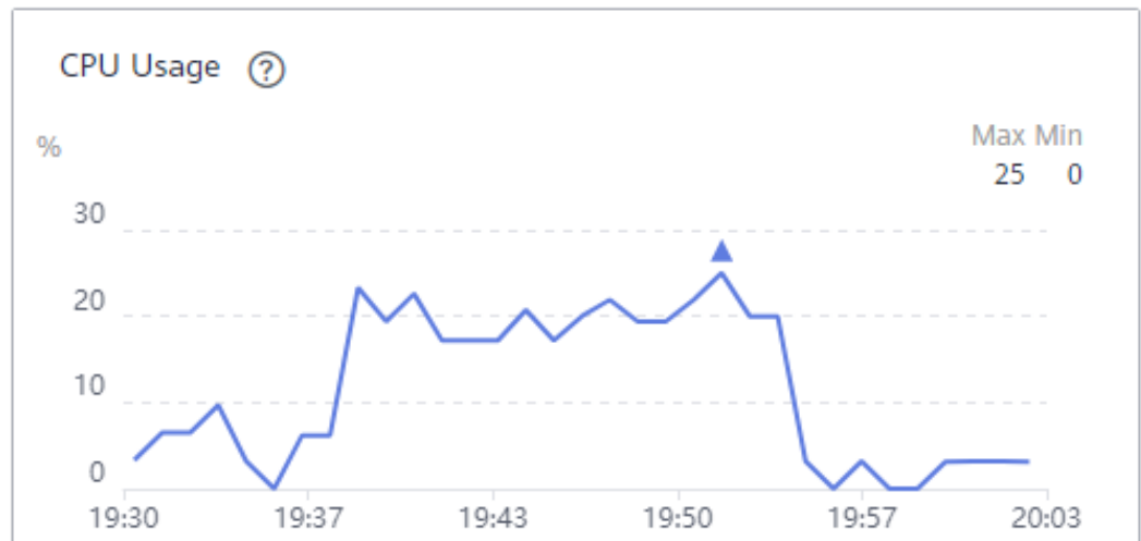
Figure 12-4 broker-1 CPU usage (batch.size = 16 KB)
