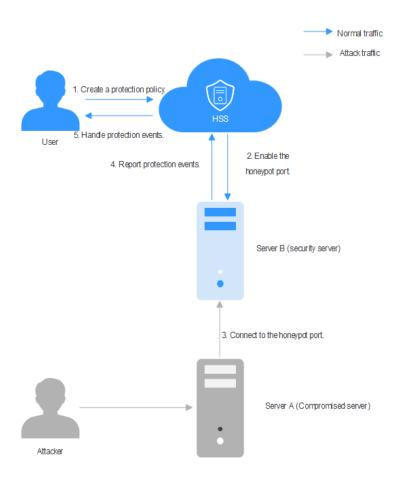
Figure 5-45 Conceptual diagram of dynamic port honeypot protection
