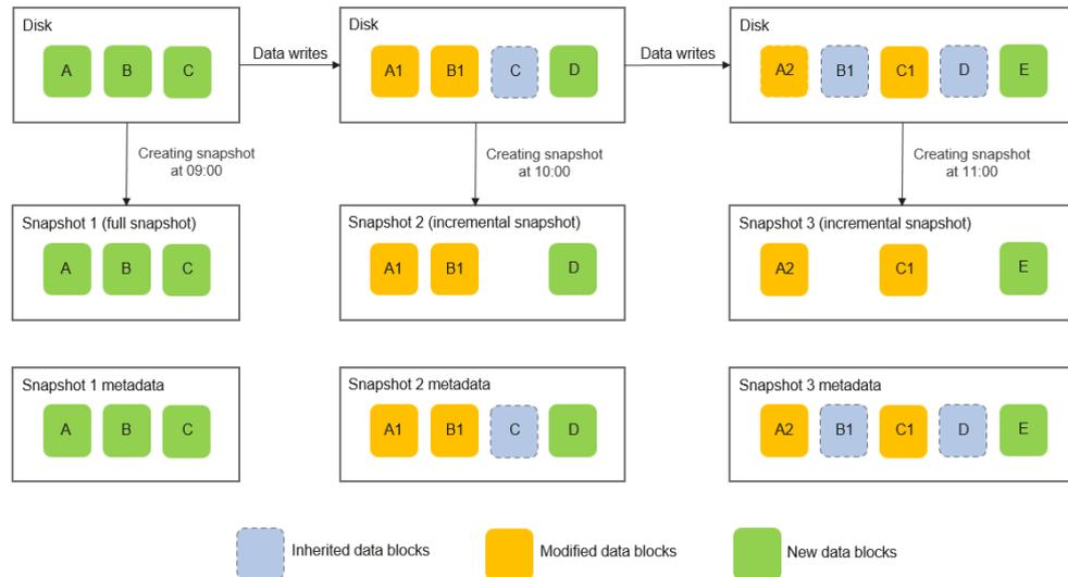
Based on the source of data blocks, a snapshot's metadata file contains information about three types of data blocks: **inherited data blocks** (inherited from the last snapshot), **modified data blocks** (have modifications compared with the last snapshot), and **new data blocks** (new compared with the last snapshot).
