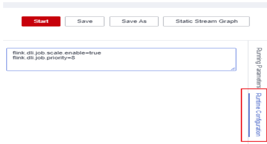
Figure 8-13 Example configuration for a Flink OpenSource SQL job
