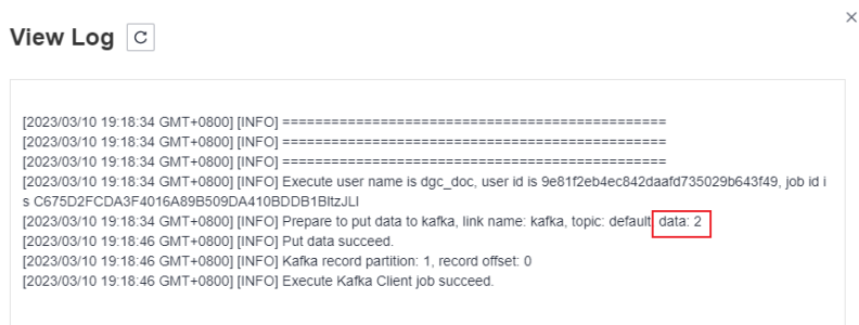
Figure 6-160 Check the Kafka Client node logs.
