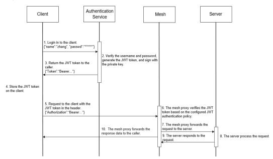
Figure 9-1 Istio JWT authentication process
