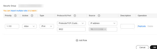
Figure 3-1 Adding a security group
