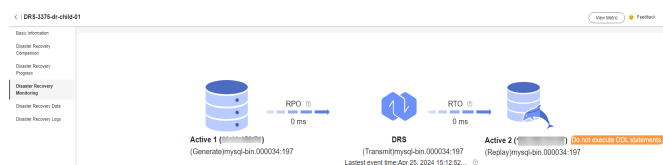
Figure 3-43 DR monitoring before direction exchange
