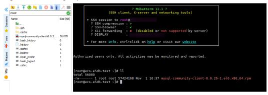
5. Install the client. rpm -ivh --nodeps mysql-community-client-8.0.26-1.el6.x86\_64.rpm
