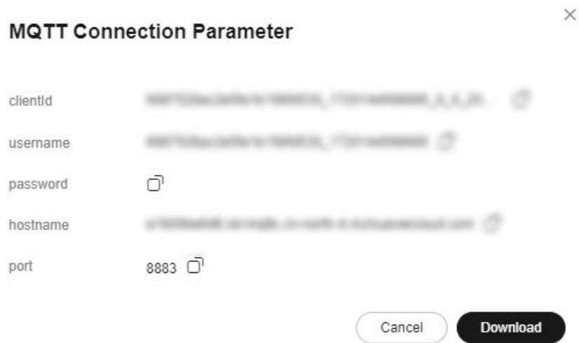
Figure 1-23 Device - Device details - MQTT connection parameters
