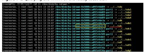
4. Stop the ECS and provide the WWN of the faulty disk to technical support personnel to replace the local disk.
