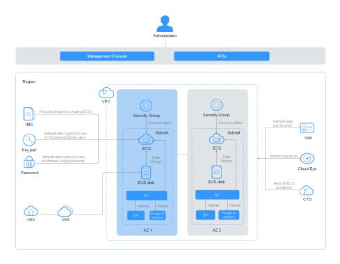
Figure 1-1 System architecture
