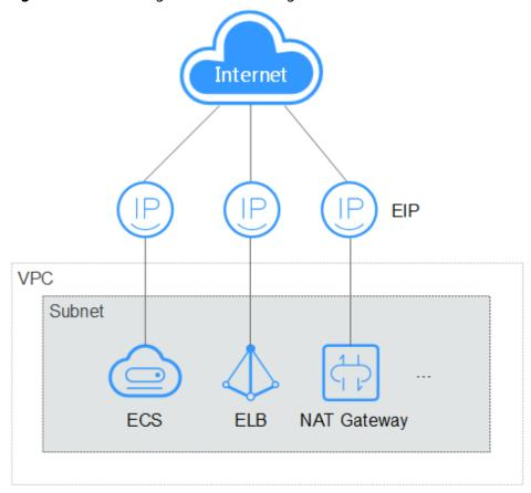
Figure 12-3 Accessing the Internet using an EIP
