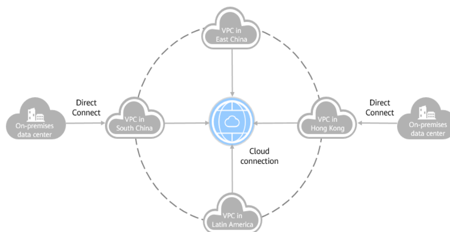
Figure 1-1 How Cloud Connect works
