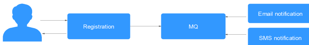
Figure 1-2 Asynchronous registration and notification using message queues
