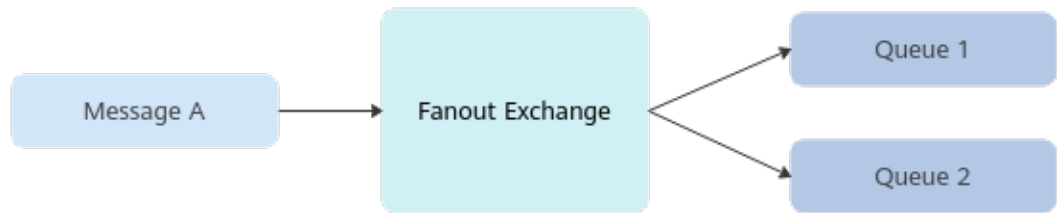
Figure 1-7 Example fanout exchange
