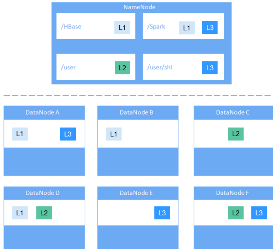
Figure 1-56 Example of label-based block placement policy
