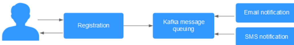
Figure 1-2 Asynchronous registration and notification using message queues
