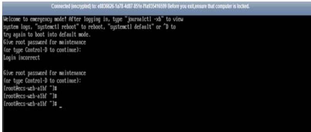
Figure 13-9 Maintenance mode of the system
