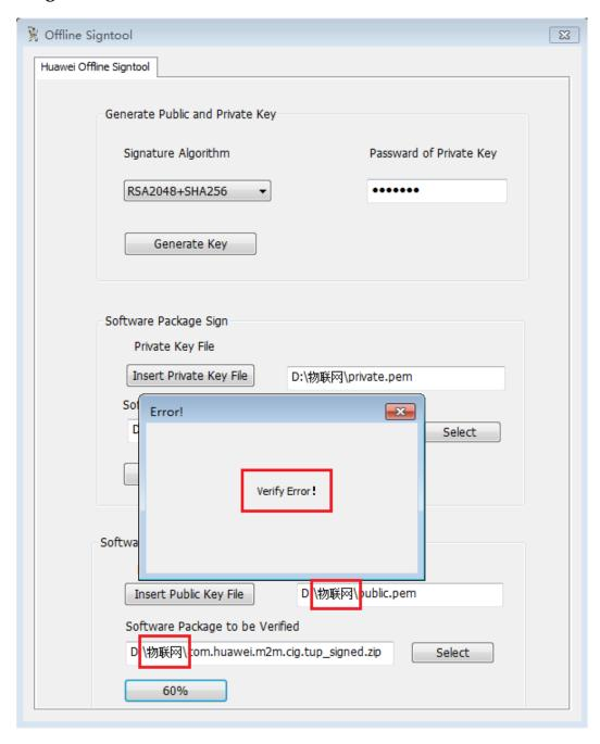
If the path of the offline signature tool or plug-in contains Chinese characters, the verification fails. Save the offline signature tool and plug-in to a path that does not contain Chinese characters.
