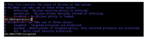
4. Open the configuration file **/etc/selinux/config**, set **SELINUX** to **enforcing**, and run the **reboot** command to restart the OS.
