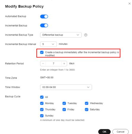
Figure 4-49 Selecting Create a backup immediately after the incremental backup policy is modified
