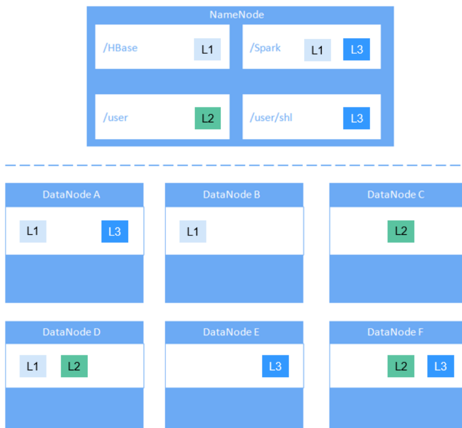
Figure 1-53 Example of label-based block placement policy
