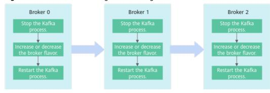
Figure 7-2 Process of increasing or decreasing broker flavors
