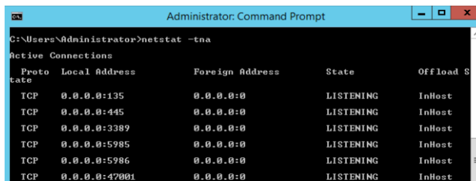
Figure 16-231 Checking network connection
