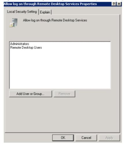
Figure 5-96 Allow log on through Remote Desktop Services properties
