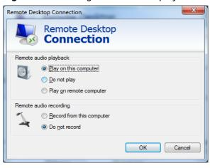
Figure 5-41 Setting remote audio playback
