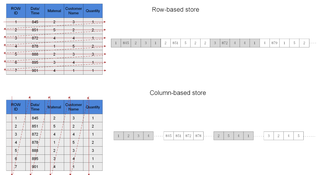
Figure 3-1 Differences between row store and column store
