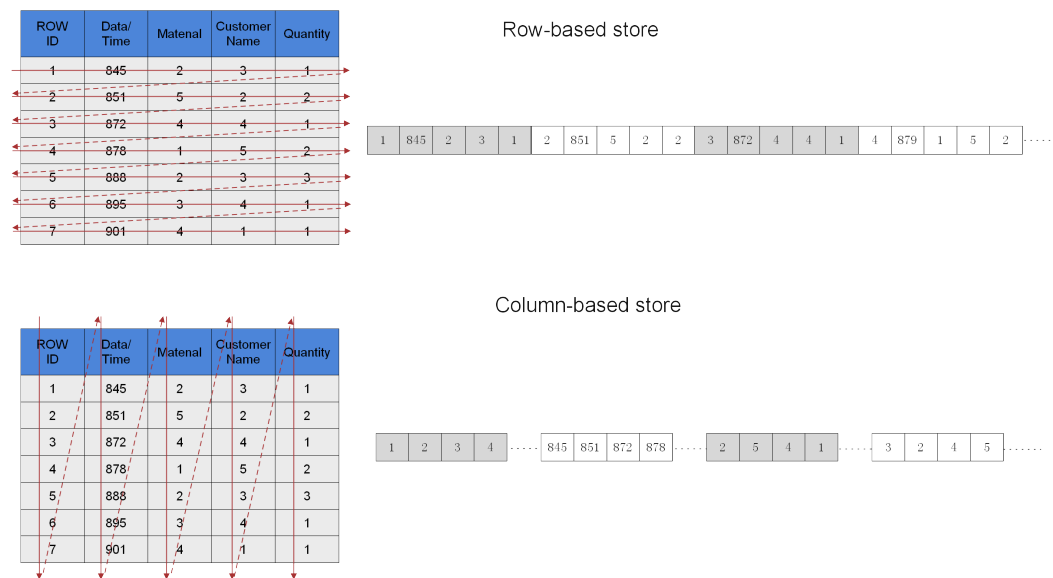
Figure 2-1 Differences between row storage and column storage
