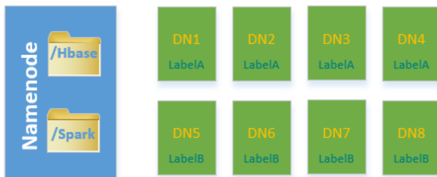
Figure 9-9 DataNode partitioning scenario
