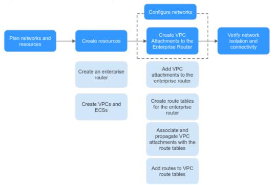
Figure 4-2 Flowchart for isolating VPCs in the same region
