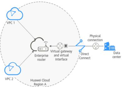
Figure 12-1 Networking between an on-premises data center and VPCs
