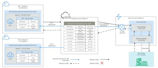
Figure 12-3 Network planning for communications between on-premises data center and VPCs
