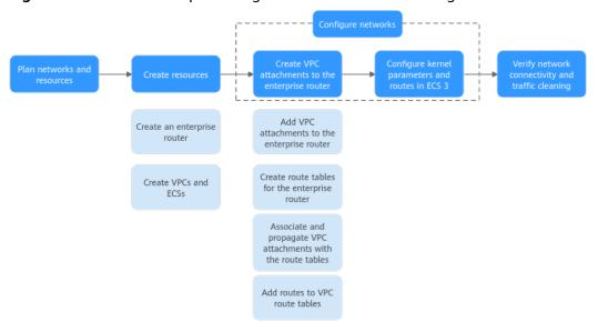
**Figure 5-2** Flowchart for protecting VPC traffic in the same region
