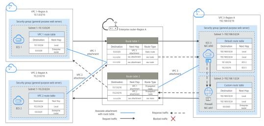
Figure 5-3 Networking planning for protecting VPC traffic in the same region
