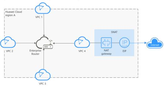
Figure 15-1 VPCs sharing an EIP through an SNAT rule
