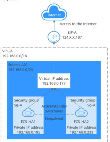
**Figure 7-6** A high-availability web cluster using a virtual IP address and Keepalived
