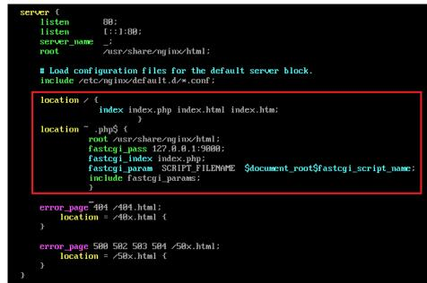
Figure 4-9 Configuration after modification
