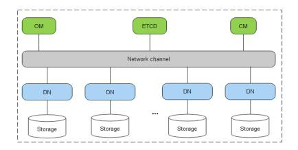
GaussDB Centralized consists of Operation Manager (OM), Cluster Manager (CM), and Data Node (DN). An application sends a task directly to the DN, and the DN returns the result to the application after processing the task.
