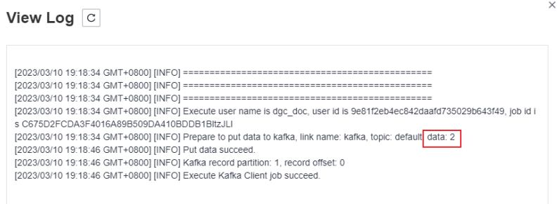
Figure 2-20 Check the Kafka Client node logs.
