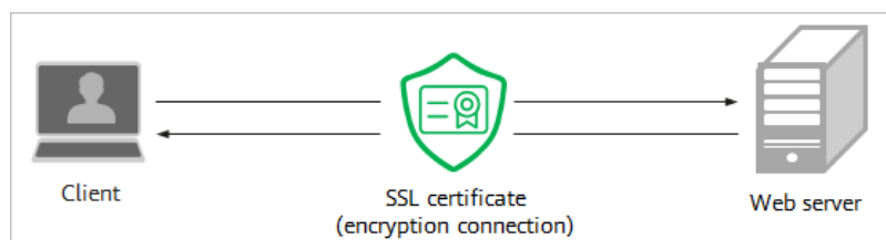
Figure 2-5 Working principles of an SSL certificate
