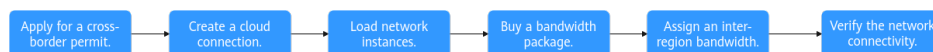
Figure 1-15 Process for connecting VPCs in different geographic regions using a cloud connection
