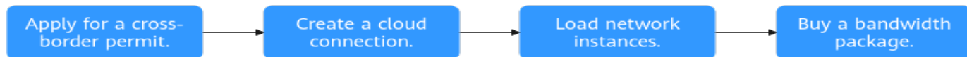
Figure 4-2 Process for connecting VPCs in different geographic regions using a cloud connection
