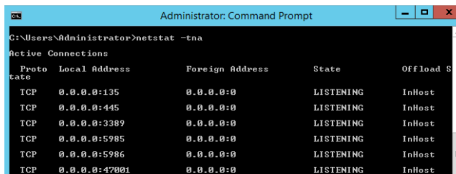
Figure 15-225 Checking network connection
