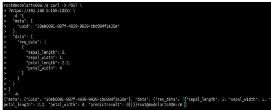
A terminal window showing the execution of a curl command to make a POST request to a deployed AI application. The command includes a JSON payload with meta and data fields, including a req\_data array with four entries. The response shows the received JSON data and a predictresult field.
