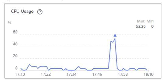
Figure 12-5 broker-2 CPU usage (batch.size = 1 KB)
