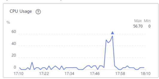
Figure 12-3 broker-1 CPU usage (batch.size = 1 KB)
