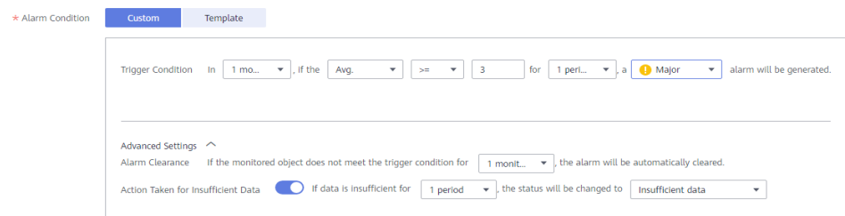
Figure 6-5 Setting an alarm condition
