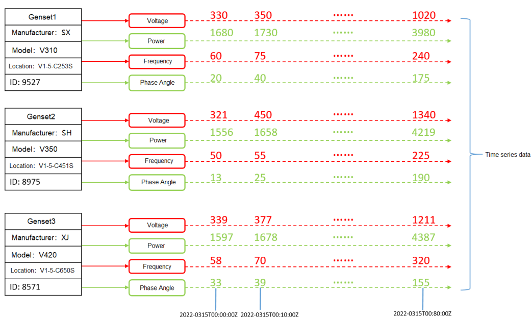
Figure 4-1 Genset data sample
