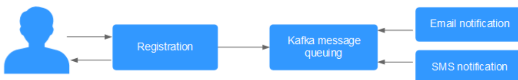
Figure 3-2 Asynchronous registration and notification using message queues
