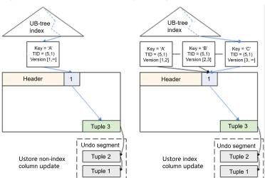
Figure 6-5 UB-tree processing during data updates
