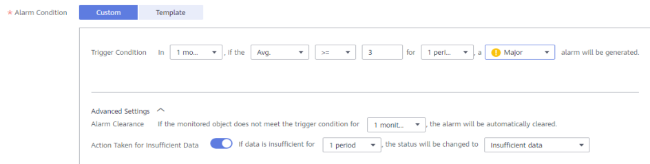
Figure 2-1 Setting an alarm condition
