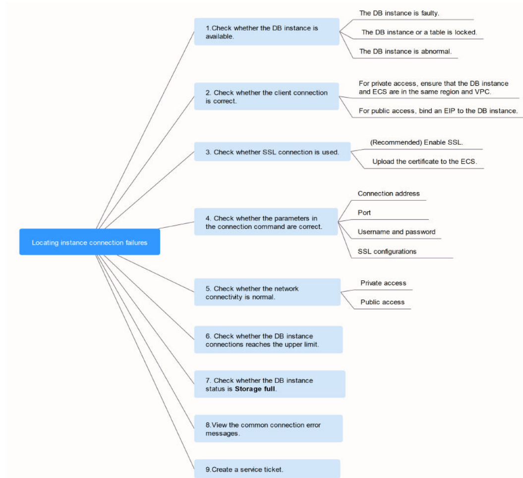
Figure 3-1 Locating instance connection failures
