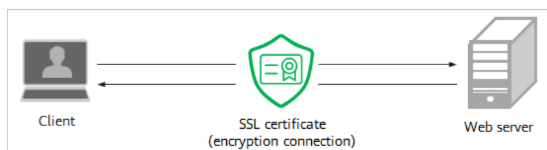
Figure 1-1 Working principles of an SSL certificate
